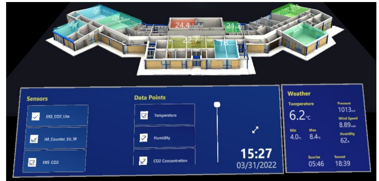
GUI showing room temperatures and desk level control panel
